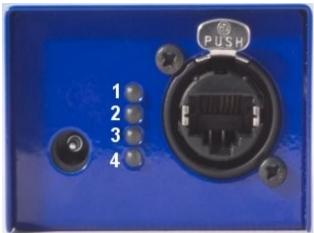
1 Status: This LED will blink when the 1 Universe Ethernet Box is operating normally. If the LED is on and does not blink it means the 1 Universe Ethernet Box is in fault, this could be due to a failed firmware upgrade. You may need to scan your network with NMU and re flash the firmware.
