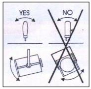
To mount on a telescopic stand (Order Code: STDTH), reverse the yoke under the fixture and bolt the stand's spigot onto the 12mm set screw.
