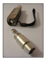
It is possible to test installed cabling using the Cable Test, by combining two devices. Place one of each of the devices on the end of the cable (you will require a female-female jumper on one of the ends) and place both Cable Tests in Cable Test mode. The test will now occur throughout the cable, and indicate any problems in the installed cabling.
