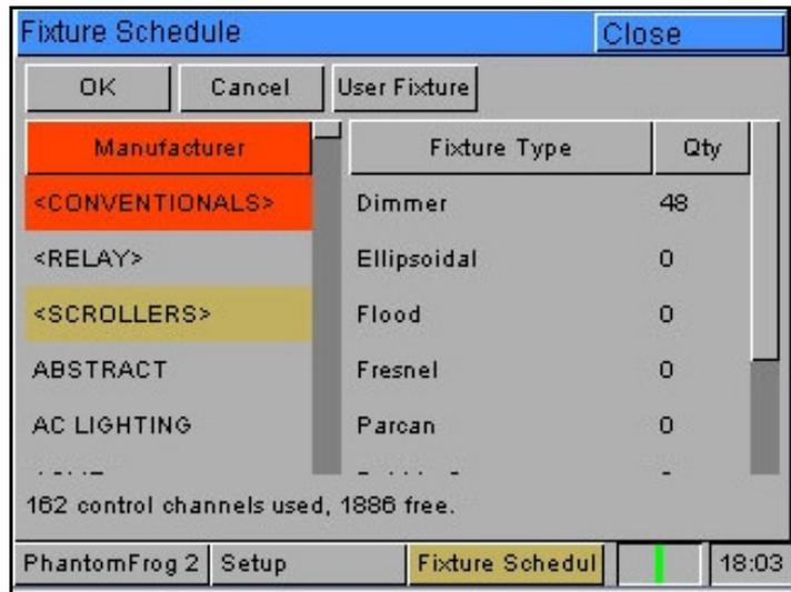
The left hand column in this screen allows you to select the fixture manufacturer.
