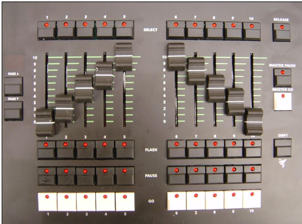
This section of the front panel contains 100 pages of 10 manual playbacks and virtual playback controls.
