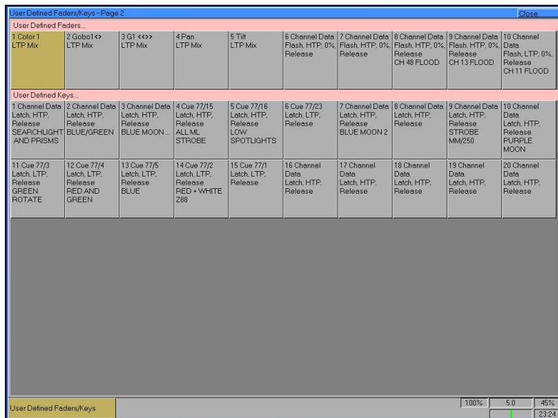
This window shows information on the current page of User Definable Faders and User Definable Keys. Each of the 20 UDK's has a button in the window. Each of these buttons shows the UDK number and information on the item assigned to the UDK (if any).
