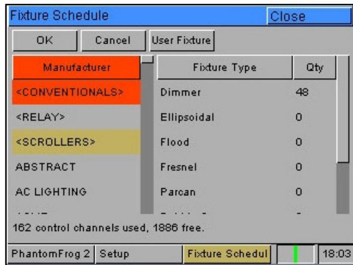
The left hand column in this window allows you to select the fixture manufacturer.
