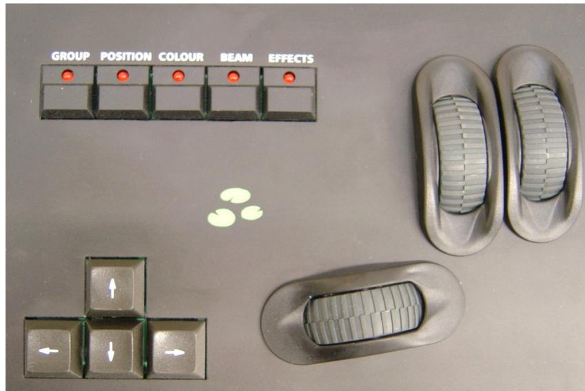
The GROUP key is used when selecting or recording groups. Pressing the GROUP key brings up a tool bar on the touch screen containing the Master Groups.
