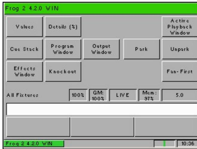
The LCD touch screen on the front panel of the desk is used primarily for displaying and selecting commonly used functions.
