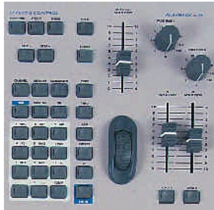
Figure 1 - 4 : Effects Controls, Numeric Keypad and Playback A/B
