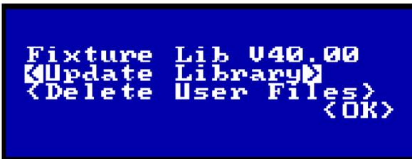
If you are currently running Zero 88 Fixture Library version 35 or later on your Jester ML or TL console, you will first need to remove the current fixture library from the console before updating to the latest fixture library. To confirm your current version, enter Setup by holding SHIFT and MODE together. Then arrow down to <Update Fixture Lib> and press ENTER. You will see the screen shown (left), with the fixture library version shown top right.
