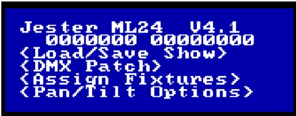
Before updating your Jester's fixture library, ensure that it is running the latest software version, which is JesterOS v4.1. To find the software version currently on your Jester, hold SHIFT and MODE together to enter Setup. The software version will be shown top right of the main LCD.
