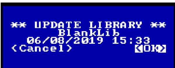
Hold SHIFT and MODE together to enter Setup. Then arrow down to <Update Fixture Lib>. Press ENTER, and then press ENTER again to choose <Update Library>. Use the Up/Down arrow keys to choose the "BlankLib" file from the USB stick, and then press ENTER to update. When Jester displays "Success", click OK. The Jester now has no Fixture Library on board.
