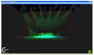
Capture 2005 visualising software communicates with the desk via a protocol known as CITP. This protocol allows for any standard PC network between the desk and the visualising PC. The console allows you to configure either a fixed IP address or one allocated via DHCP. As long as the two devices can see each other, the system should function correctly.
