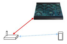
With a PC connected to the network with the desk and the PDA, load up an internet browser and type in <a href="http://192.168.0.1/">http://192.168.0.1/</a> (or the configuration IP address of the router, if different) into the address bar and hit GO.
