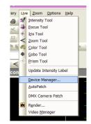
In Device Manager, select New and locate the Zero 88 console you are connecting to
