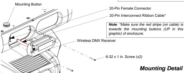
Figure 2: Wireless DMX Receiver Installation
