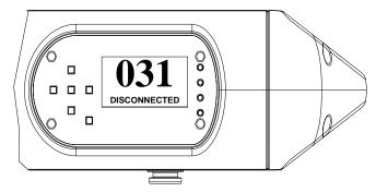
Figure 7: LCD Display - Disconnected Screen
