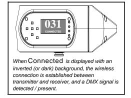
Figure 5: LCD Display - Connected Screens
