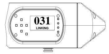
Figure 4: LCD Display - Linking Screen
