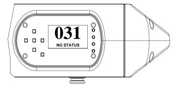
Figure 6: LCD Display - No Status Screen
