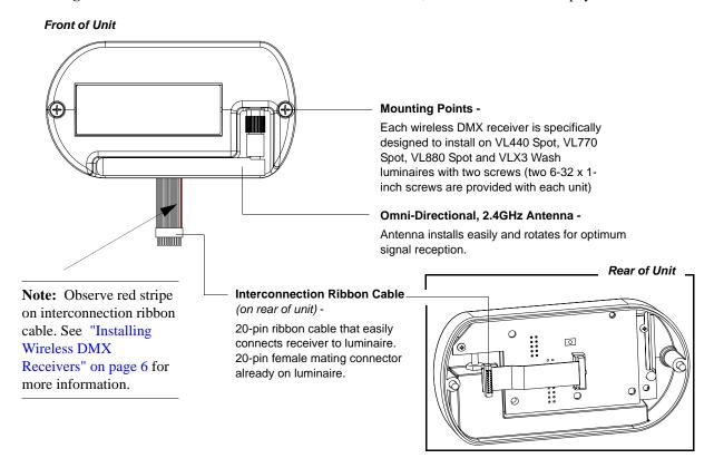
**Figure 1: Wireless DMX Receiver Features**
