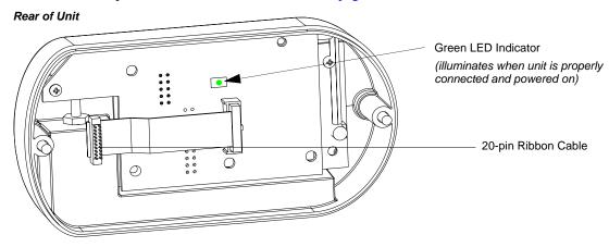
Figure 8: Green LED Indicator (Rear of Wireless Receiver)
