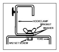
To mount on the theatre standard scaffold pipe (48mm O.D.) use a theatre hook clamp (G clamp) (Order Code: 20HC). Your luminaire is supplied with a 12mm set screw, washers and a nut. Thread the set screw through the yoke from the inside, put on a washer, then the hook clamp, another washer and then do up finger tight with the nut.
