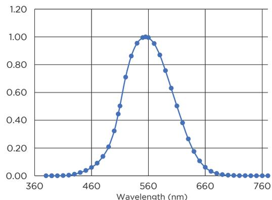
**FIGURE 1. EYE SENSITIVITY CURVE ACCORDING TO CIE**
