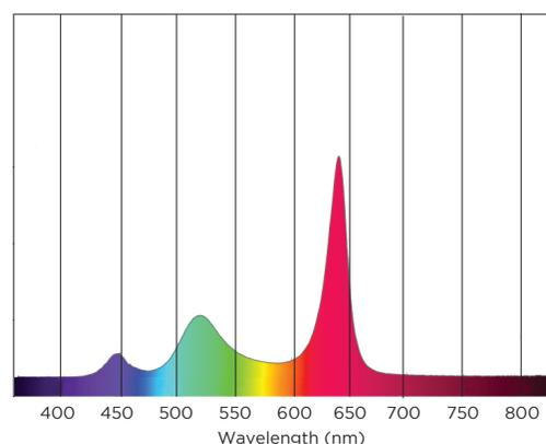
**FIGURE 7. RGBW FIXTURE AT 3000K WHITE**
