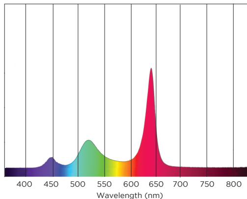
**FIGURE 7. RGBW FIXTURE AT 3000K WHITE**
