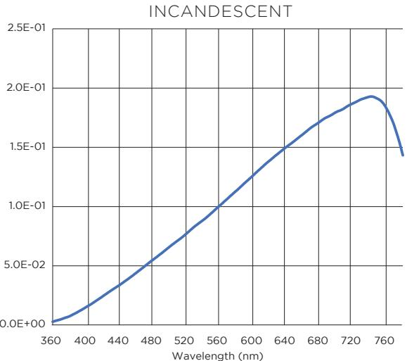
FIGURE 2. INCANDESCENT FIXTURE SPECTRUMS
