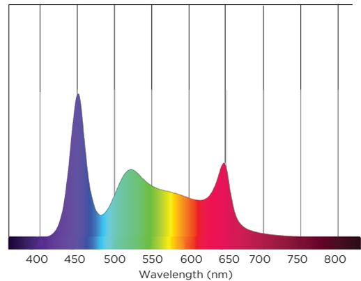
**FIGURE 15. VLS LED PRODUCING 8000K WHITE**
