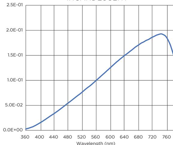
**FIGURE 2. INCANDESCENT FIXTURE SPECTRUMS**
