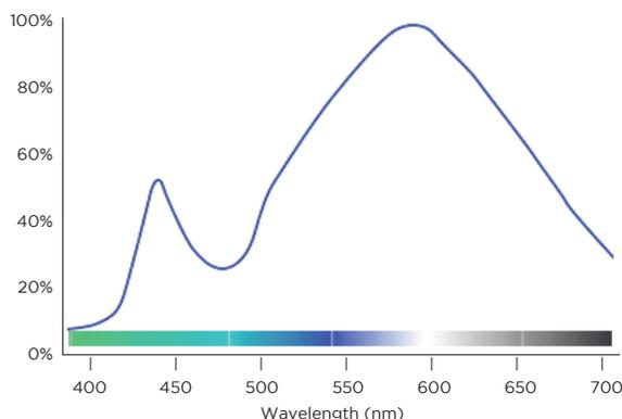
**FIGURE 6. SPECTRUMS OF TYPICAL WHITE PHOSPHOR LED<sup>2</sup>**
