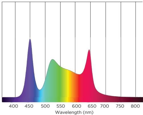
**FIGURE 14. VLS LED PRODUCING 5600K WHITE**
