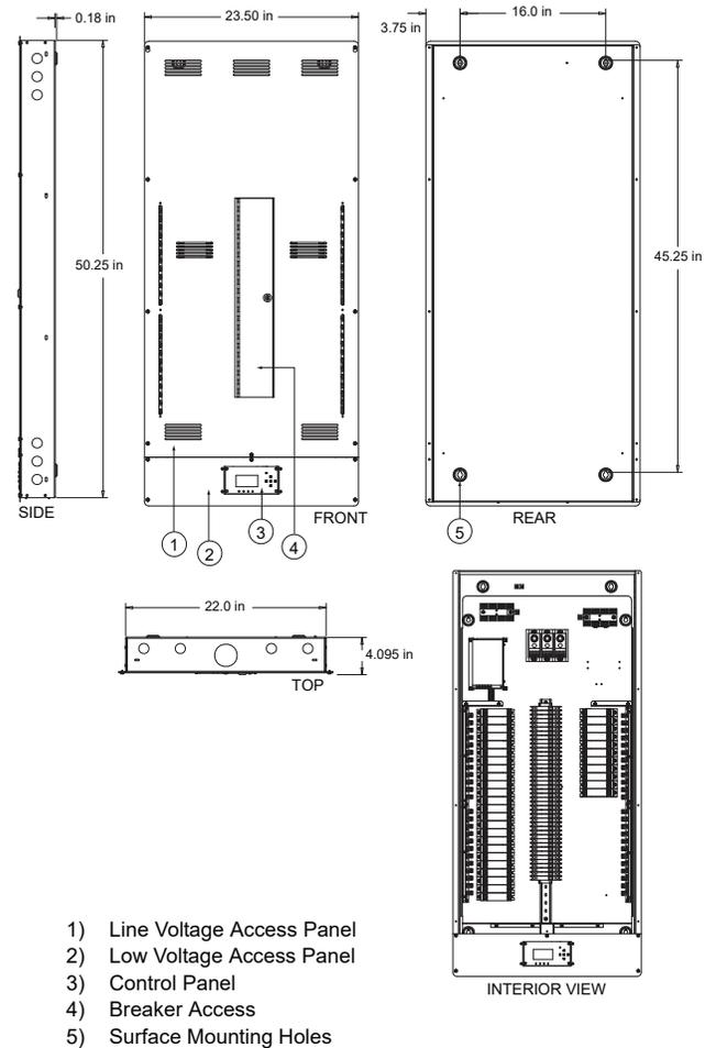
**48-WAY RELAY INSERT PANEL W/ BREAKERS (76923C)**
