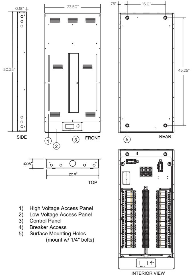
**42-WAY RELAY INSERT PANEL W/ BREAKERS (76933C)**
