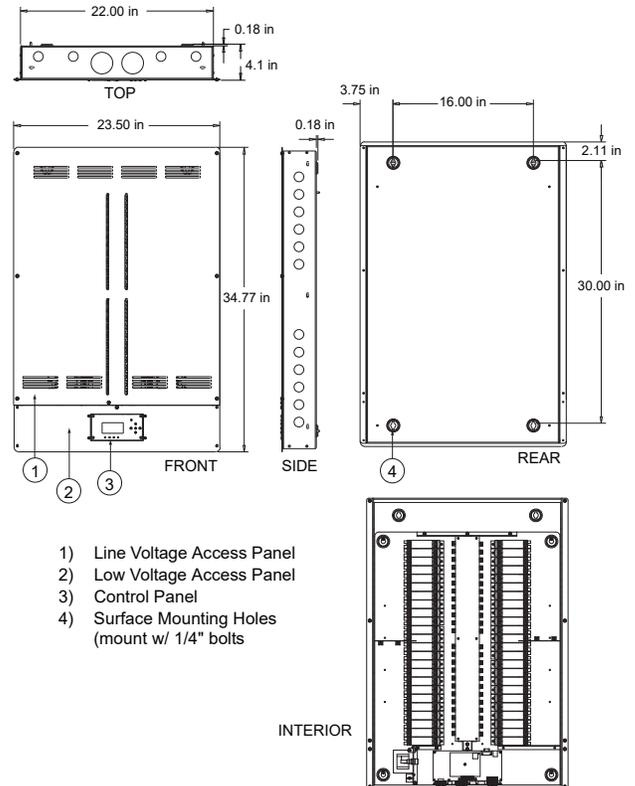
**24-WAY RELAY INSERT PANEL W/ BREAKERS (76921C/76931C)**
