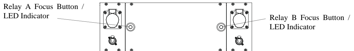
Figure 3: Relay Module Focus Buttons / LED Indicators
