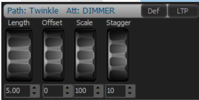
**Length:** How long the FX runs before it starts over. **Offset:** Low value. **Scale:** Hi value. **Stagger:** applies a delay to the start of each channels level change. Once set, this can be recorded into a cue or recorded as an FX for later playback. To record into a cue, press [RECORD] [#] [ENTER] and make sure the “FX” identifier is yellow. This will include FX in any cue recording.
