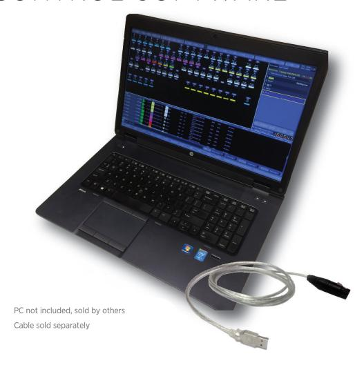
NEO PC allows all the same functionality from the powerful NEO software to output from your own PC whether you use the optional USB to DMX Cable or an existing DMX Ethernet network.
