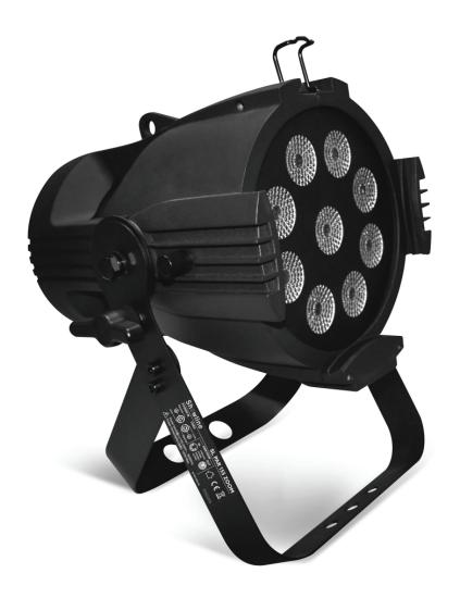
The SL PAR 155 ZOOM is a die-cast aluminum LED Par can that utilizes nine homogenized RGBW LEDs to produce over 3200 lumens of output. The manual zoom provides a beam angle range from 80 to 400 and the split yoke bracket allows for easy hanging or floor mounting.
