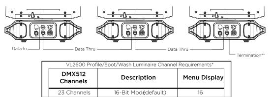
\*\*DMX terminator required for last fixture on DMX line.
