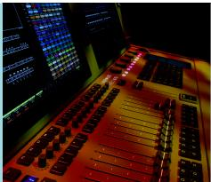
The Neo X15 is Vari-Lite's flagship, high-performance lighting console designed for large facilities, and helps designers find the perfect look in less time with an advanced effects engine that supports pixel mapping, media playback, timelines, and more.
